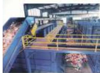
Left: Example of automated sort line found in state-of-the-art single stream material recovery facility (MRF)
